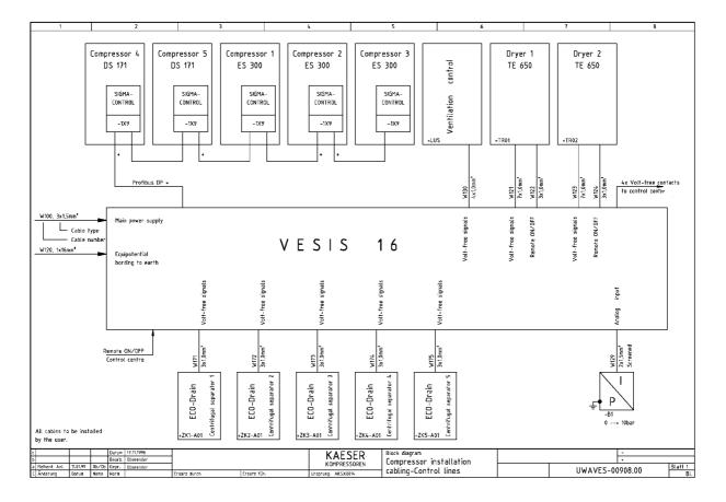
Wiring of the process field bus with the help of the above circuit diagram
