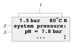
1 Current system pressure and airend discharge temperature
