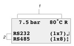
1 Current system pressure and airend discharge temperature
