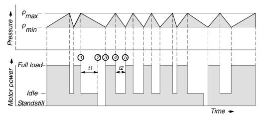
In DUAL control mode (combined idle and start-stop) the compressor normally runs in **load** and **idle** or **standstill**.
